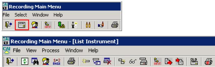
To display a list of instruments, click the List Instruments icon from the toolbar. From this screen you can add new instruments, locate and display instruments, and print reports as described below. Lien instruments, which have been released by other referred instruments, will be displayed in yellow. Also, instruments which have been referred to, or referred by other instruments will have check marks in the *Refers To* or *Refers By* columns.
